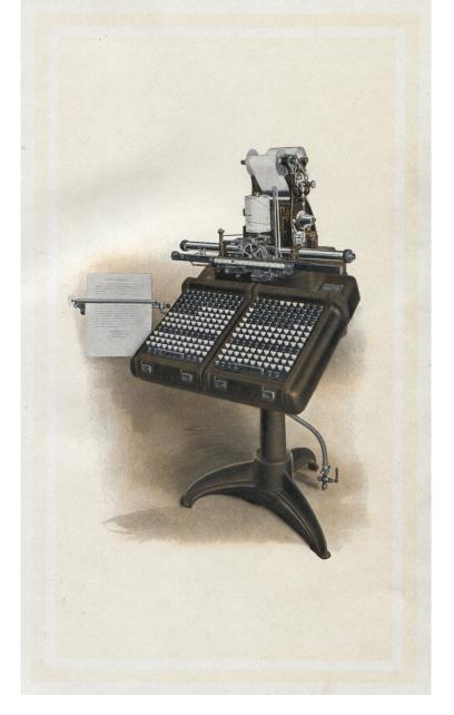
was, not surprisingly, used to enter text. As an operator keyed in copy, the key codes were punched onto the paper tape, along with spacing information. Rich Hopkins describes it well:
